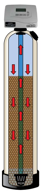
**Hellenbrand Neutralizing Filter** – This system is recommended for pH adjustment for waters with pH 6.0 - 6.9. Typical signs of low pH are blue green stains. The system uses a self sacrificing media which has to be refilled periodically.
